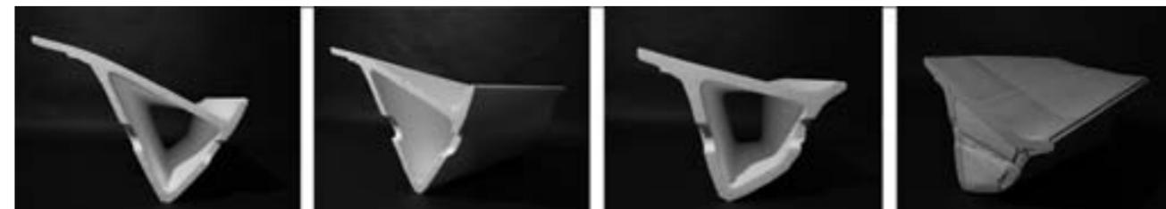
7 Full-scale voussoirs—wire-cut EPS (left) and cast concrete (right)
