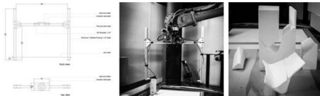
6 Wire cutting tool and initial cutting tests
