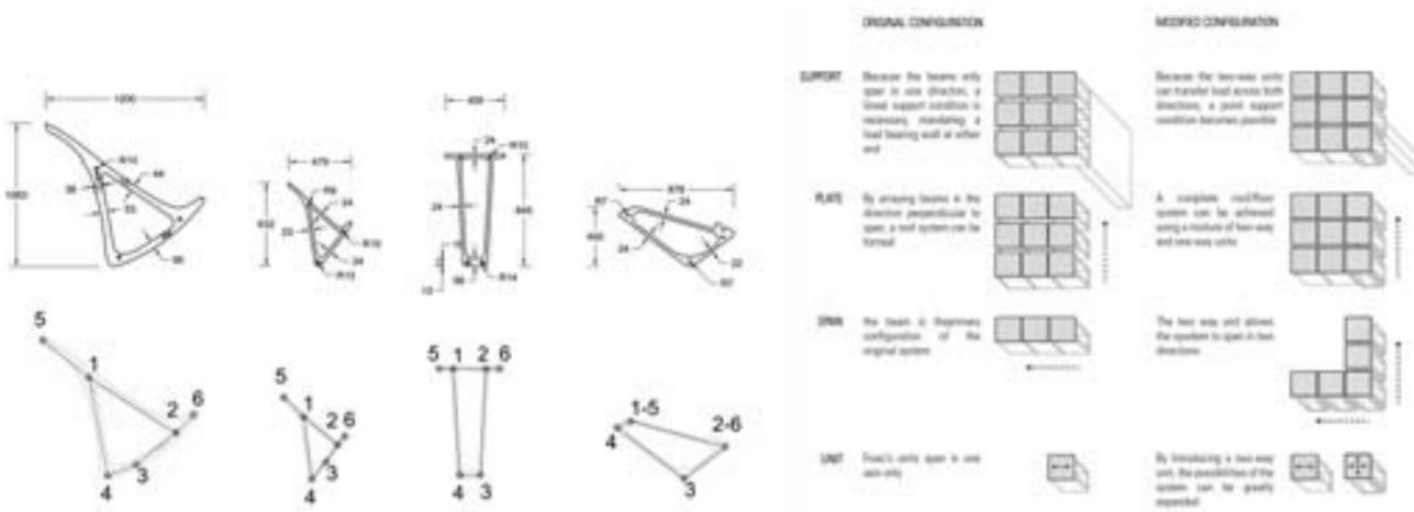
3ab Left: Parametrization of the “bones” series’ six control points; Right: Topological variation by introducing a girder unit
